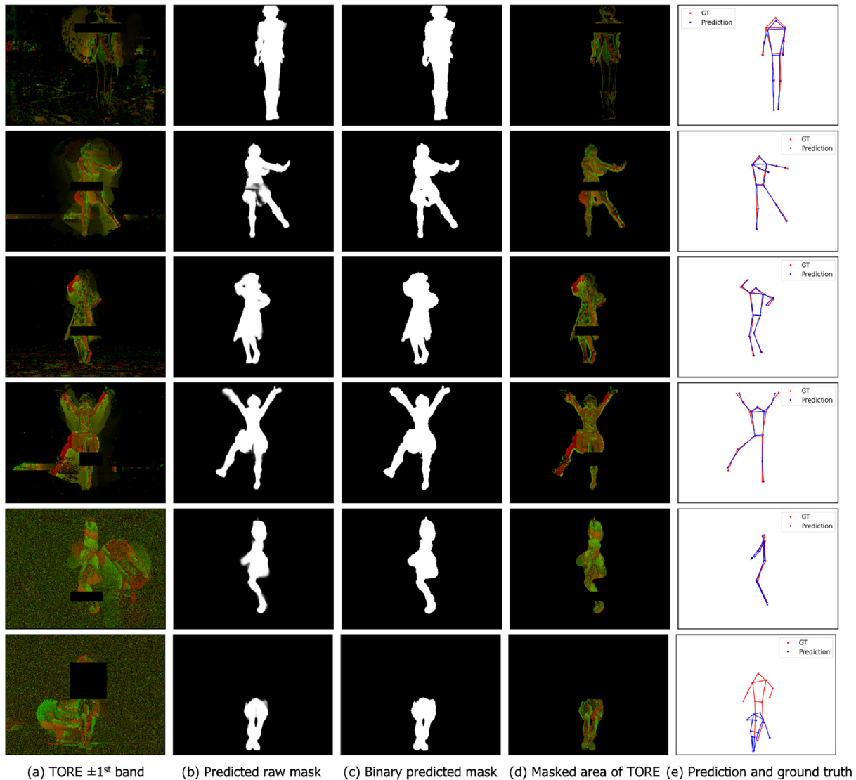
Fig. 11. Samples of occluded inputs, predicted mask, TORE volume representation, and inferred human poses.
